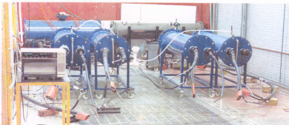
Load cycling in water 2 bar water pressure
